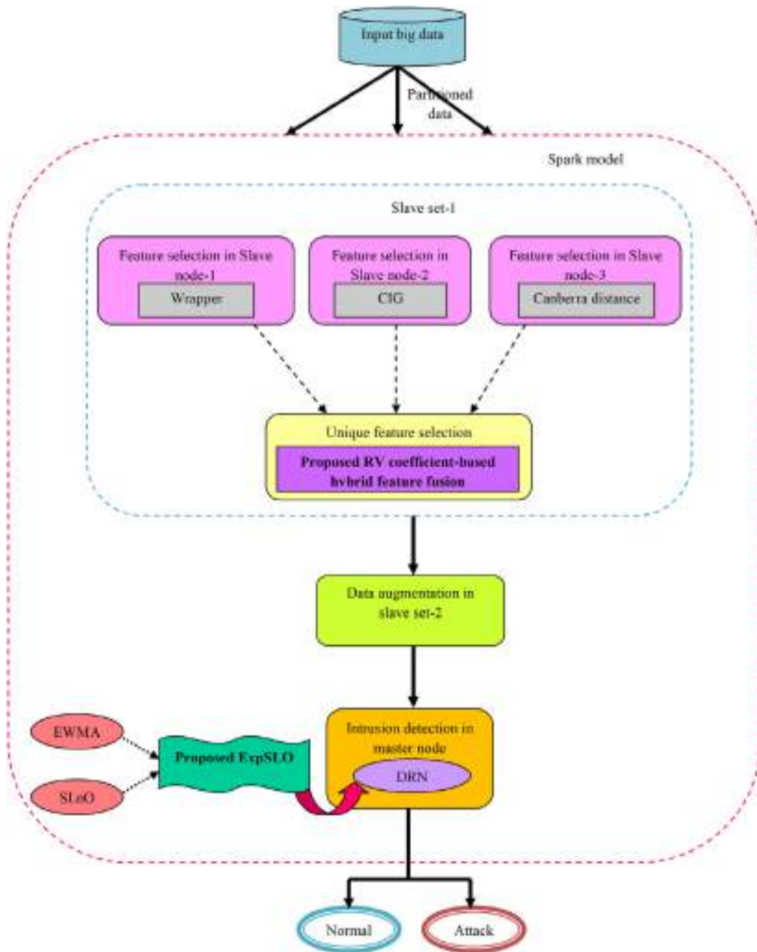
Fig. 1. Schematic representation of the developed RV coefficient+ExpSLO-based DRN for the intrusion detection.
